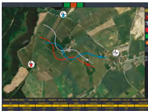
Figure 4. An example of improper operation of the system due to azimuths misalignment. The system detected and was tracking three objects instead of one.
