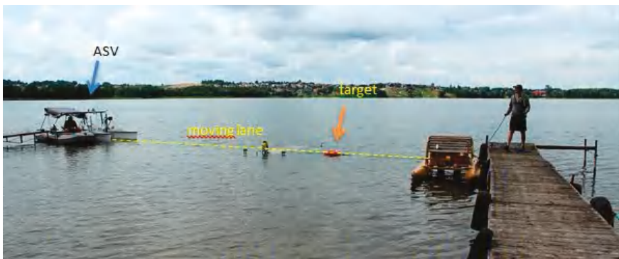
Figure 4. Configuration for stationary research. Targets were moved along the “moving lane” in front of the stationary HydroDron.
