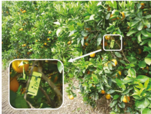
Figure 4. Location of the acceleration sensor on a fruit-bearing branch on the outermost part of the canopy.
