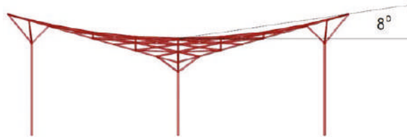
Figure 6. Determination of the roof inclination angle.
