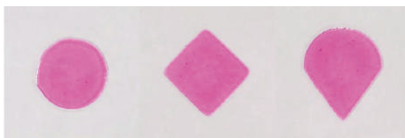
Figure 5. Stencil printed discs of 3 geometries using ink formulation HPMC 16% (500 μm stencil height).
