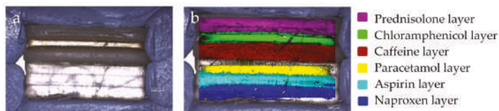
Figure 3. Visual imaging of a Type I polypill, using (a) optical light microscopy and (b) Raman mapping. The images show the spatial separation of layers.
