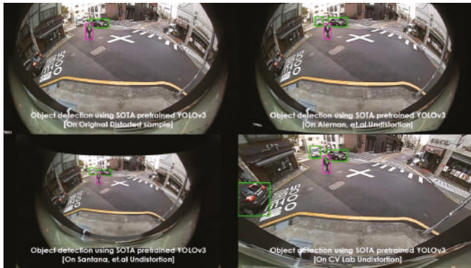
Figure 11. Pretrained YOLOv3 object detection on various rectified 190° fish-eye frames: car detected along the edge in the proposed rectified algorithm.
