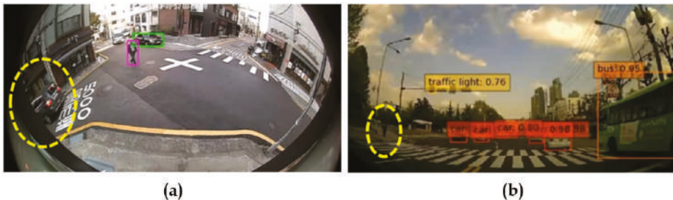
Figure 8. Performance of pretrained state-of-the-art (SOTA) models on different larger FOV raw samples: (a) Pretrained YOLOv3 on 190^\circ fish-eye sample (car undetected along the edge); (b) Pretrained SSD on 120^\circ wide-angle sample (person undetected along the edge).
