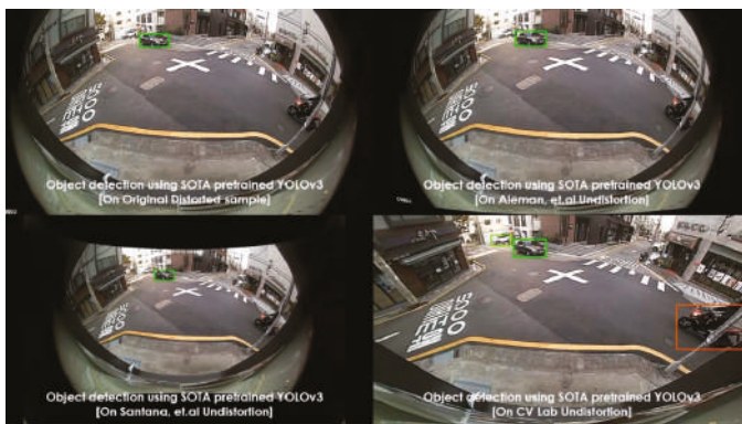
Figure 13. Pretrained YOLOv3 object detection on various rectified 190° fish-eye frames: motorbike detected along the edge in the proposed rectified algorithm.
