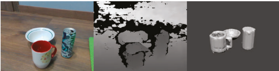
Figure 15. An example of reconstruction of multiple objects in the scene: segmented and classified RGB frame (left), depth frame (middle), and predicted depth mask (right).
