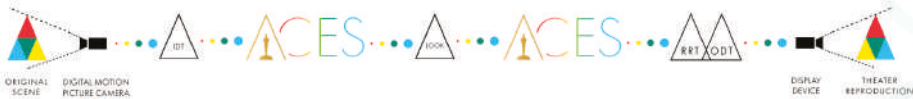
Figure 10. Schematic of a linear and very simple ACES color pipeline; the black-edged triangles indicate ACES components. Left-to-right: Camera footage enters ACES scene-referred colorimetry via an IDT; creative color decisions are applied as Looks (LMT); final output is carried over through the Output Transform (RRT + ODT) combination, leading to a display-referred colorimetry ready for output to standard output device (a theatrical projector in this case).
