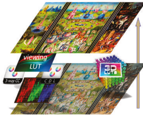
Figure 3. Toy-model of a simple, single-camera, non-ACES “basic” grading pipeline: the arrow on the right orders the “layer-based” representation of real-time image processing operations, as performed by the color-correction system in the background, while colorist works. Source footage in its camera-native colorimetry ( bottom ) is creatively modified by color transforms, either coming from the set (Color Decision Lists, cfr. Section 2.4) and applied in-theater (3-way CC’S); then a “viewing LUT” is applied on top to match the colorimetry with the output device’s for viewing ( top ). A 3D LUT may represent the overall effect of a single primary grade (possibly lacking accuracy [17,20]), and may include the viewing LUT and all color-space conversions (courtesy: Hieronymus Bosch, The Garden of Earthly Delights , c.1495–1505).
