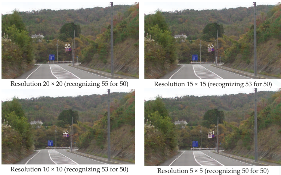
Figure 19. Example of recognition results for 50 km speed-limit sign.
