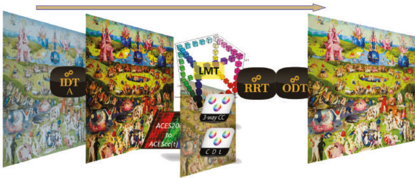
Figure 15. ACES-based color grading (cfr. Figure 3), with the arrow on top ordering this “layer-based” representation of real-time image processing. Source footage in its camera-native colorimetry (left) technically enters the color pipeline by means of Input Transforms (camera A is represented, but different IDTs may be used for cameras B, C, ...). After everything is converted in ACES2065-1 CVs, creative grading is done via same operators as in the non-ACES case, i.e., CDLs, 3-way CC’s, creative LUTs (both LMT and secondary grades), with implicit conversion to either ACEScc or ACEScct as working color-space and, after all CC layers, back. Viewing on the reference monitor/projector (right) is done via RRT + ODT (courtesy: Hieronymus Bosch, The Garden of Earthly Delights , c.1495–1505).
