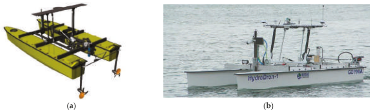
Figure 5. Combined skid and traditional steering system—motors and rudder design plan (a), photo of USV HydroDron during experiments (b).
