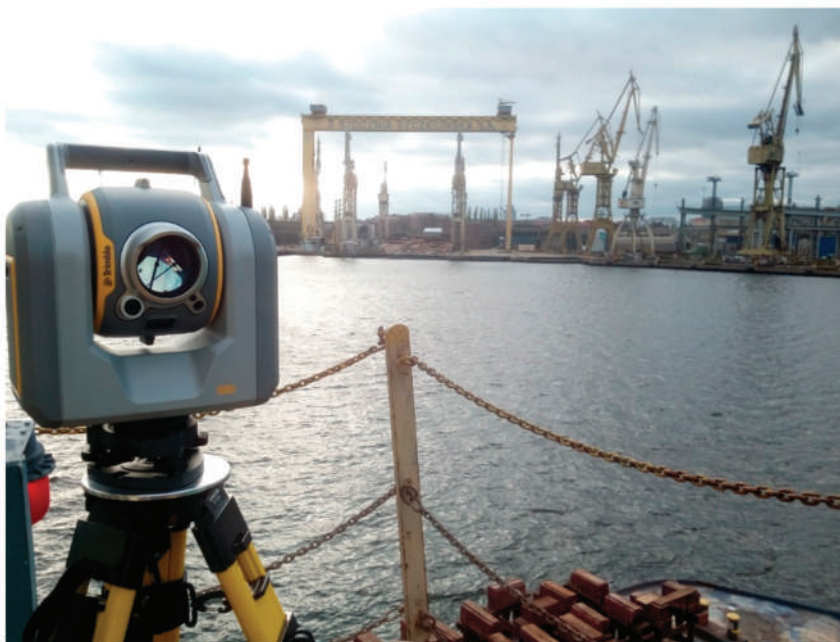
Figure 7. Total station measurements on a tilted reference frame (on the ship in the water).
