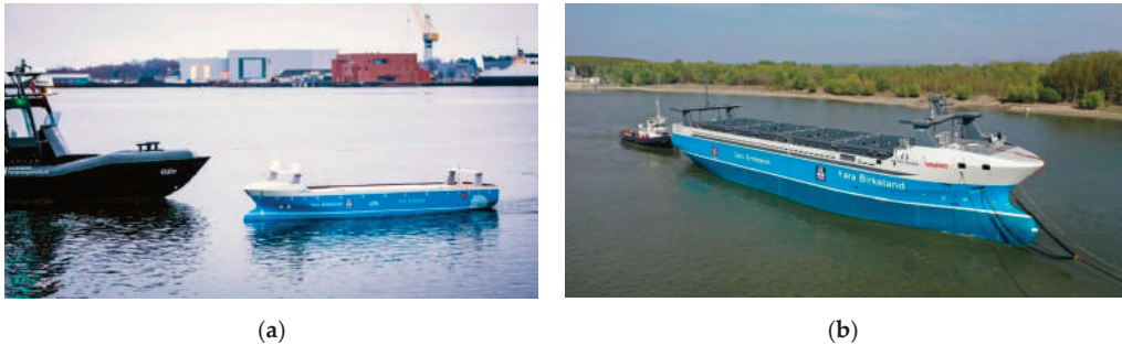
Figure 1. Model of the ship Yara Birkeland for research and testing (a) [9], and the autonomous container ship Yara Birkeland launched in February 2020 (b) [10] (120 TEU, L = 79.5 m, B = 14.8 m).
