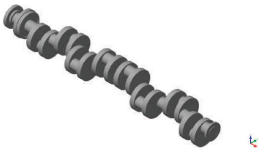
Figure A4. A 3D model of the crankshaft S-12075-3600-10-8-149-144-C-04.
