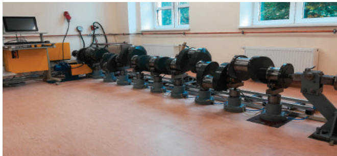
Figure 2. The test rig operating in line with the concept of the measuring system with flexible support of a crankshaft (own source).
