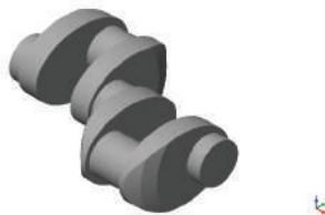
Figure A10. A 3D model of the crankshaft S-1977-0740-3-2-149-144-O-10.
