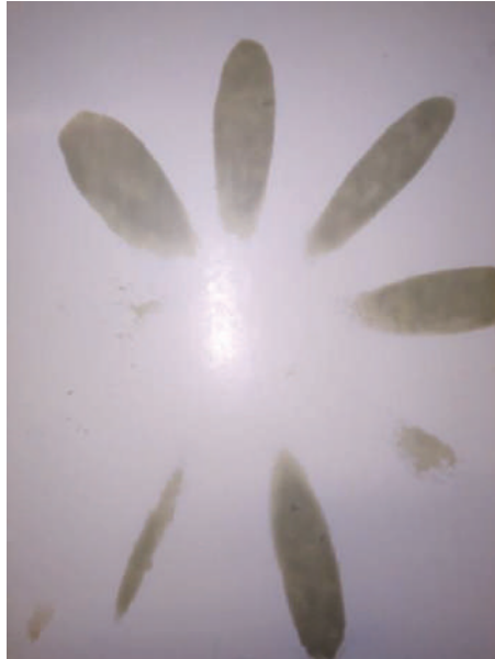
Figure 4. Fuel stream sprayed by a coked injector nozzle (naturally coked obtained from the engine department of the repair shipyard). Three out of nine ports are clogged.
