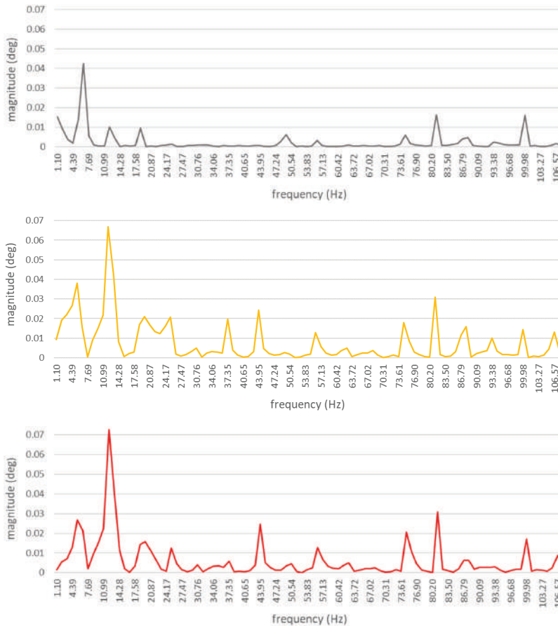
Figure 13. Absolute values of differences in the spectra related to a diesel–electric unit with a defect-free engine and with a defective injector nozzle. The diagram is limited to the 16th harmonic component only. Waveforms for: differences between defect-free and first coked; differences between defect-free and second coked; differences between defect-free and third coked.
