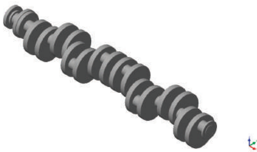
Figure A3. A 3D model of the crankshaft S-16942-3600-10-8-149-144-C-03.
