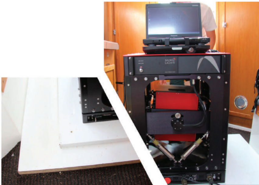
Figure 3. MGS-6 mounted on the survey vessel. On the left is shown how the frame was fitted to the deck using thick chipboard plates.
