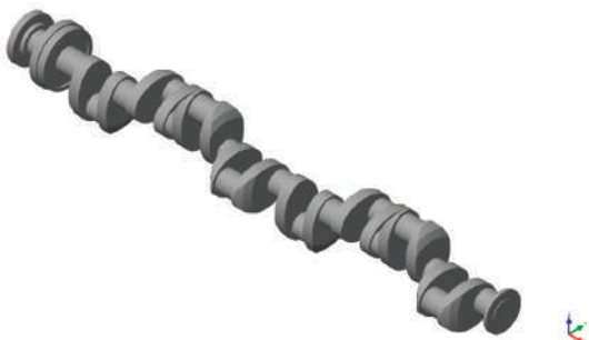
Figure A5. A 3D model of the crankshaft S-9283-3600-10-8-149-144-O-05.
