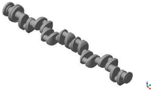
Figure A2. A 3D model of the crankshaft S-8658-3600-10-8-149-114-O-02.
