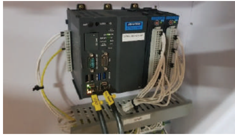
Figure 2. Data collection system in Voyage Data Recorder (VDR).
