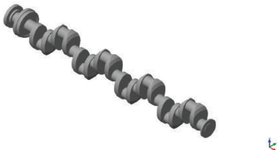
Figure A6. A 3D model of the crankshaft S-9283-3600-10-8-149-144-O-06.
