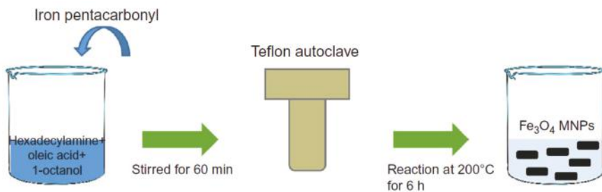
Figure 4. A schematic describing the hydrothermal synthesis approach. The process is similar to the co-precipitation; however, after preparing the mixture, the solution is transferred to an autoclave for further aging at high temperature and pressure for several hours [26].
