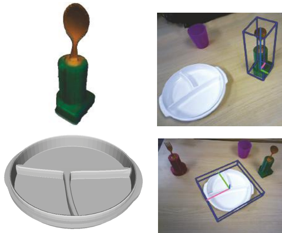
Figure 8. Qualitative results visualisation of the estimated pose of two project objects. The spoon model was scanned and the plate was modelled.
