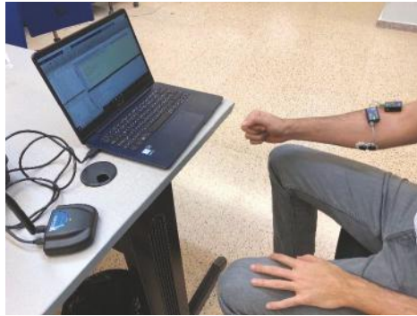
Figure 2. Surface electromyography (sEMG) system acquiring data from a subject.
