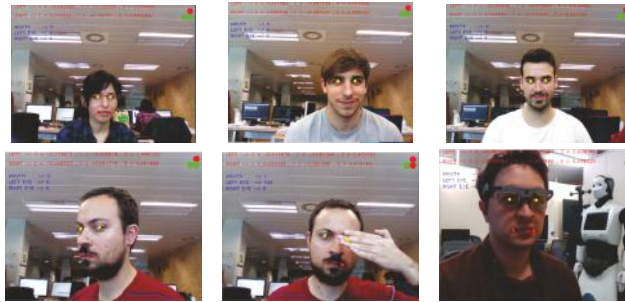
Figure 9. Qualitative results visualisation of the estimated mouth pose with five users. Red points are the mouth landmarks and yellow points the pupil landmarks. The top-right circles indicate if the user has their mouth or the eyes open (green) or closed (red) (best viewed in colour).
