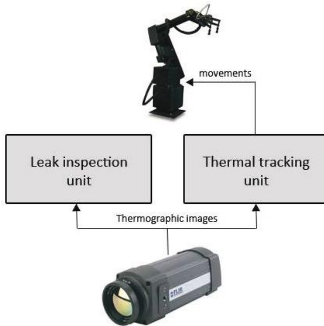
Figure 3. Software architecture: leak inspection unit and thermal tracking unit.
