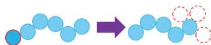
Figure 1. Schematic of the reptation move implemented through a configurational bias pattern with n_{\text{trials}} = 3 . Different candidate positions could be picked by the selection of the bond length, bending, and torsion angles used for the re-configuration of the monomer.
