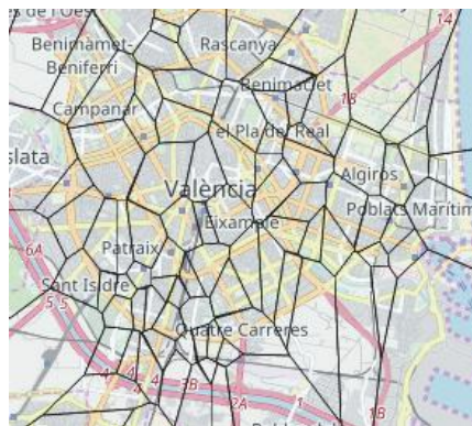
Figure 3. Voronoi diagram from the selected zones as potential points to locate charging stations.
