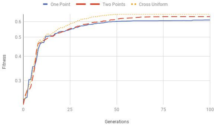
Figure 7. Maximum fitness values for different crossover techniques with an initial population of 2000.
