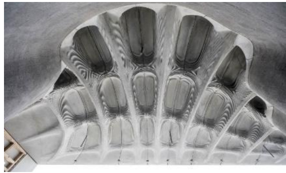
Figure 5. Concrete part formed on a Binder-Jetted tool [38].
