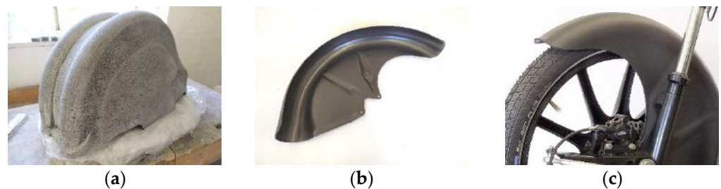
Figure 15. (a) Binder-jetted sand mold for thermoforming thermoplastic fenders, (b) thermoformed fender made from ABS, (c) application of the ABS fender.
