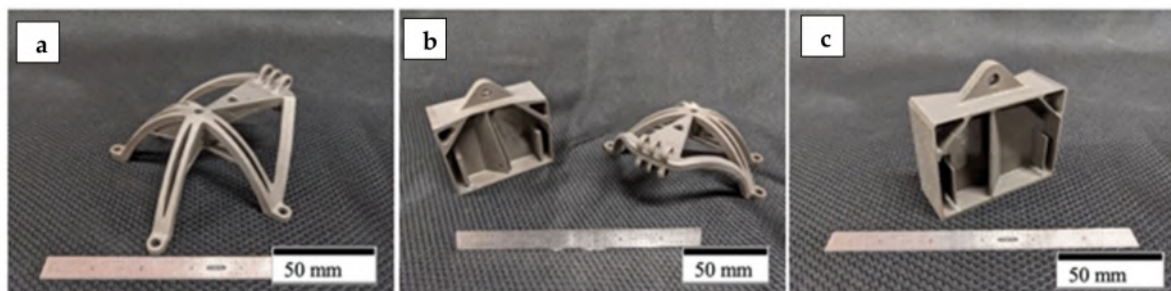
Figure 4. Annealed parts successfully printed from Ti64 HDH. (a) Topologically optimized bracket. (b) Side to side printed geometries. (c) Electronics box enclosure.
