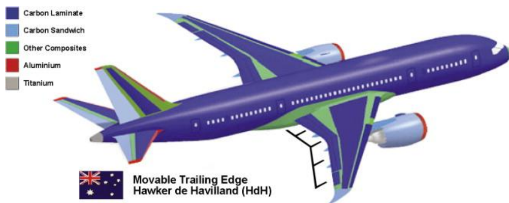
Figure 5. Material utilization in the Boeing 787 Dream Liner manufactured by HdH [24] (reprinted with kind permission from Elsevier).
