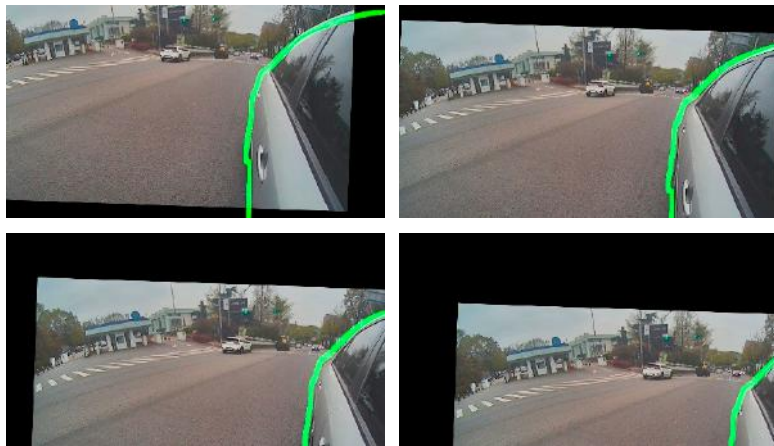
Figure 22. Calibrated images corresponding to Figure 21, where the green lines denote the boundaries of a 3D vehicle model image.
