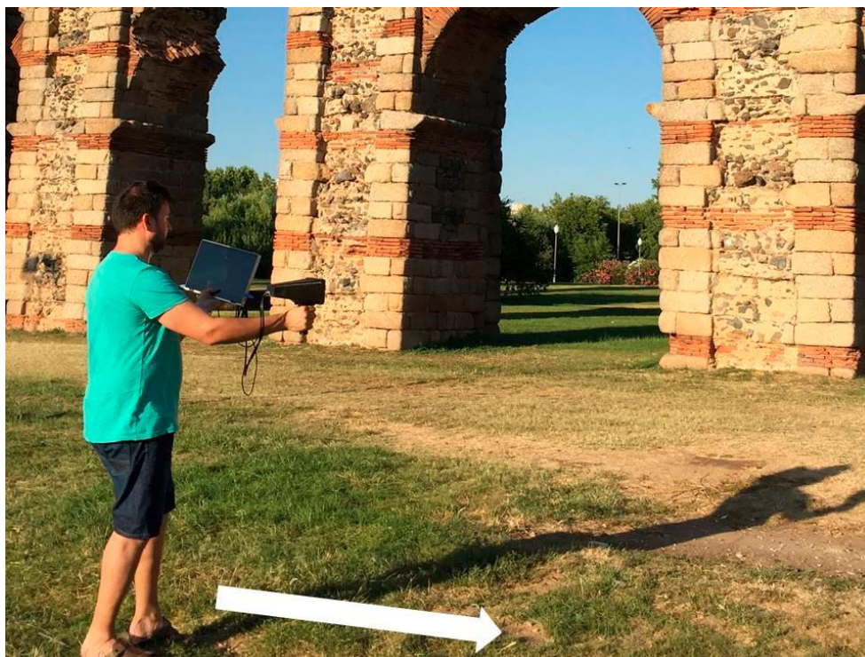
Figure 2. In-field data capture. The white arrow indicates the user direction movement, parallel to the monument façade, followed during this test.
