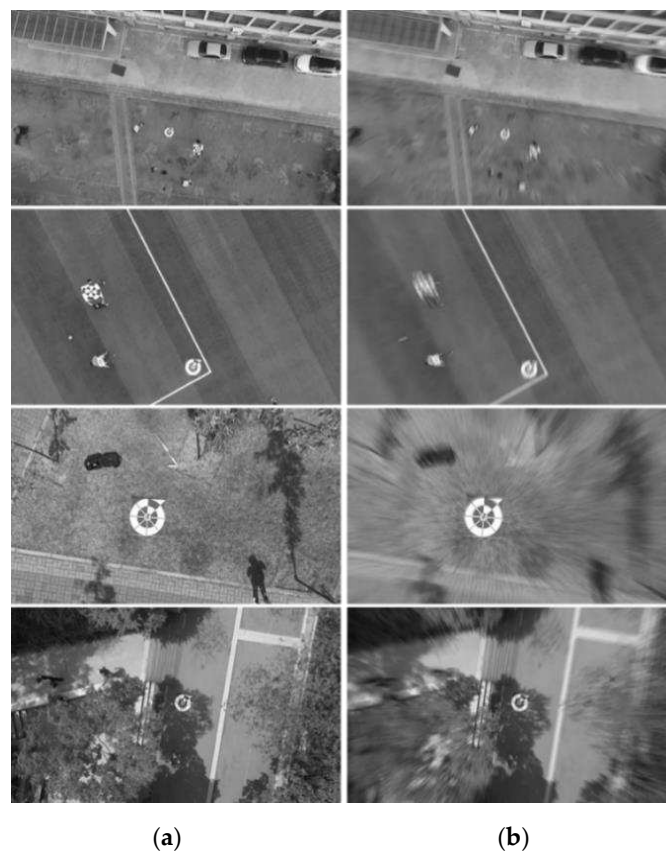
Figure 6. Examples of RMBD-DB1. (a) Ground truth (original images), and (b) motion-blurred images.
