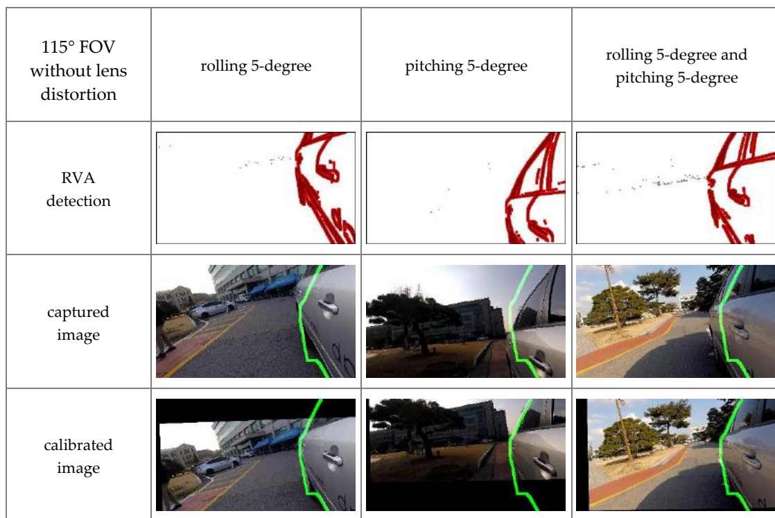
Figure 19. Experimental results with 115-degree FOV camera and lens distortion correction in different orientation conditions, where the green line denotes the boundary of the 3D vehicle model.
