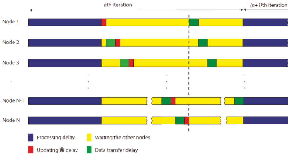
Figure 6. Timing diagram of the processes carried out by each node of the network at each block iteration.
