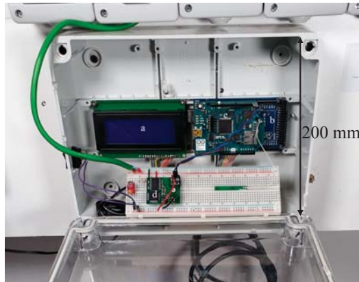
Figure 13. The low-EB prototype and a the liquid crystal display (LCD); b: the Arduino Mega 2560; c: the WiFi shield; d: the sim Tapko and e the shielded twisted pair (STP) cable.
