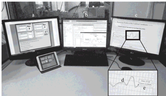
Figure 12. The aggregator; a: graphic-user-interface; b: Matlab; c: power flow monitoring at the point of delivery; d: actual power flow; e: forecast power flow.
