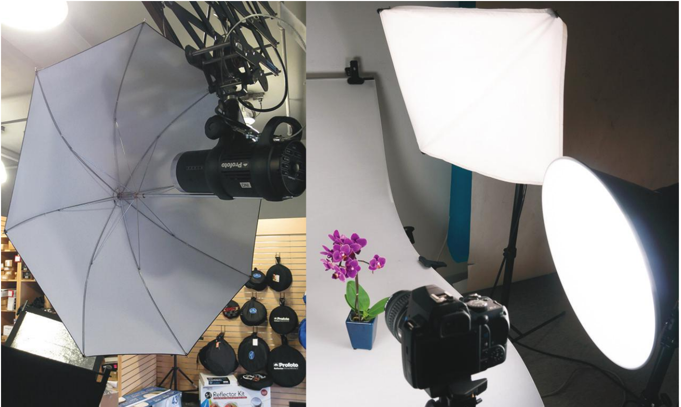
Figure 2-9. Studio lights with umbrella reflectors (left) or soft box diffusers (right) help illuminate still-life, product, and portrait shots with soft, even lighting.
