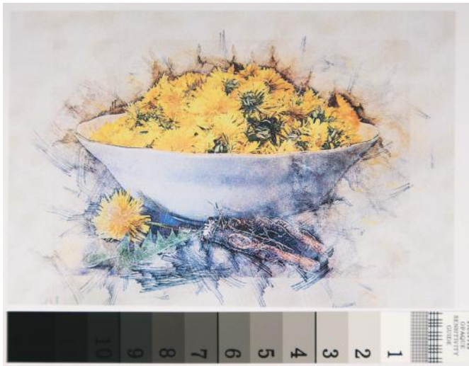
Figure 5-2. Copy photo with a grayscale included with the subject for later use in setting highlight, midtone, shadow, and gray balance.
