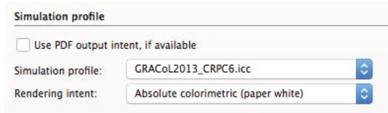
Figure 4-6. Simulation profile in EFI’s Fiery RIP. The simulation profile enables an inkjet proofer to print color that looks like it came from a lithographic press printing to GRACoL specifications. (GRACoL stands for General Requirements in Applications of Commercial Offset Lithography.)
