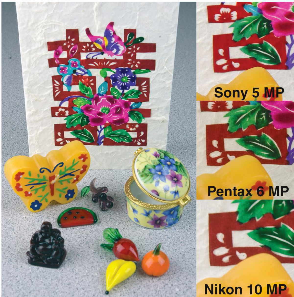
Figure 2-2. The same still-life scene was photographed with (A) a 5-MP point-and-shoot camera, (B) a 6-MP DSLR, and (C) a 10-MP DSLR. A small square in the image was then cropped to a size of 1.6 in. at 300 ppi. Differences in camera resolution are apparent in the relative sizes of the cropped areas. Also, slight differences in color rendition are visible among the cameras.
