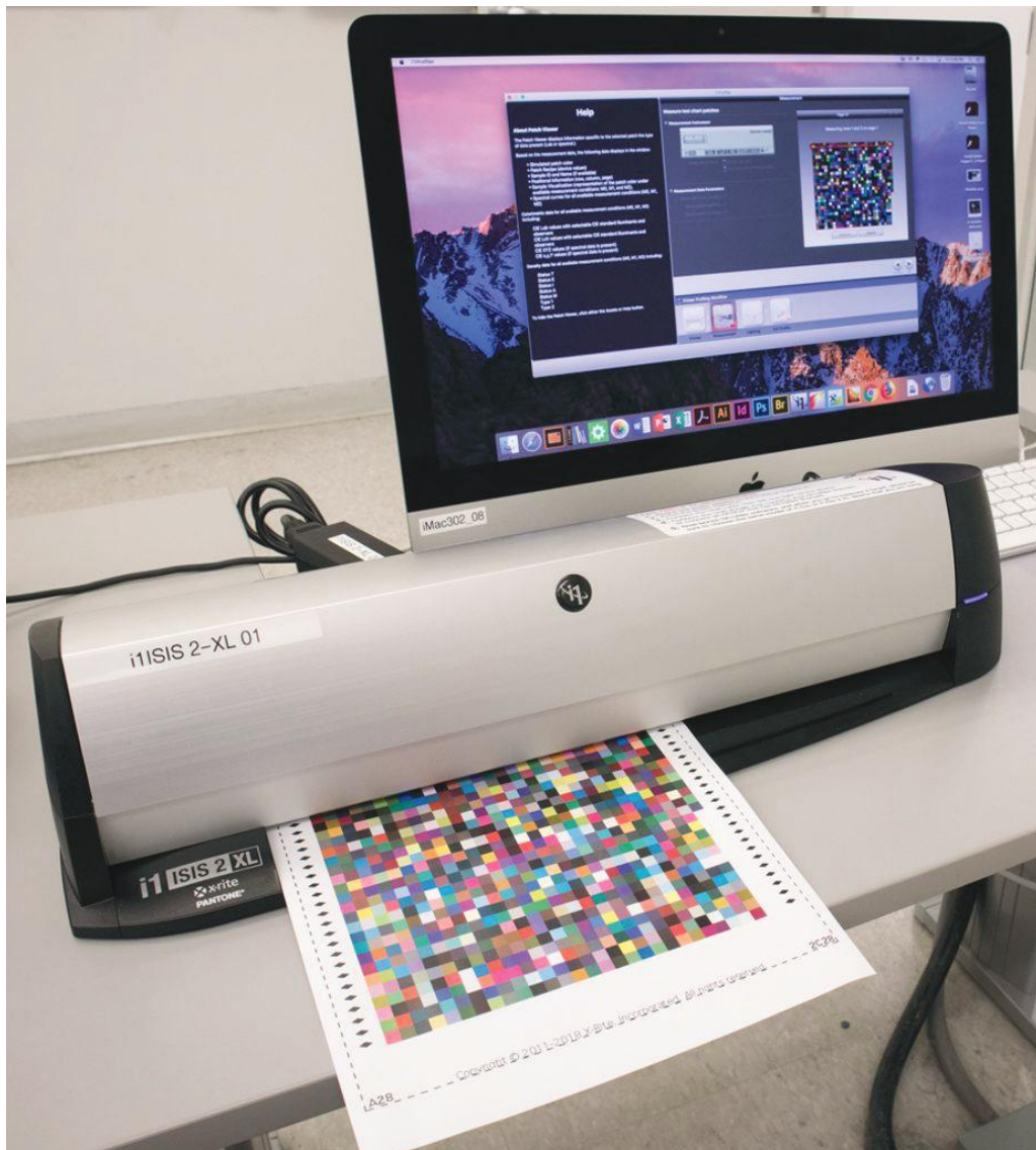
Figure 4-13. A printer profile is made with an i1 iSis x/y-scanning, or fully-automated, instrument. The instrument reads the set of 800 patches unattended in about 4 min.
