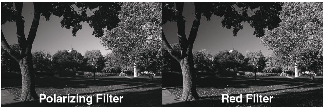
Figure 2-8. Comparison of grayscale photos taken with a polarizing filter (left) and red filter (right). The red filter darkens greens and blues in the scene, increasing contrast.
