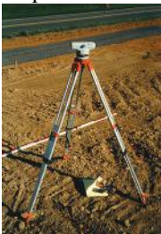
A level used for determining elevations.
